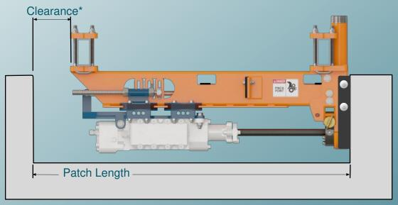
\* 7" Clearance for a 12" hole depth with 48" patch length
